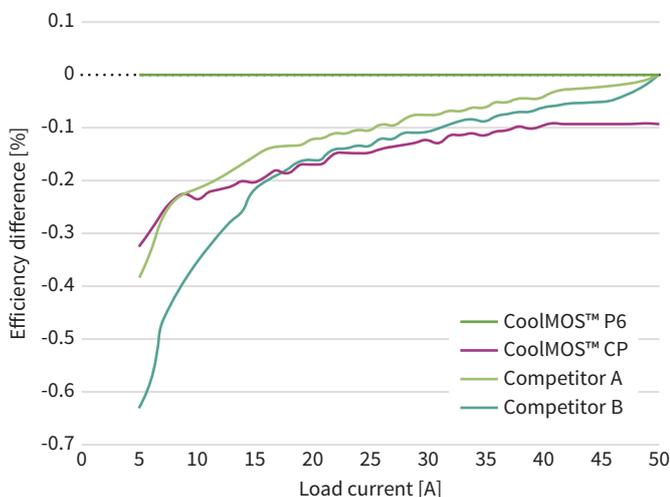
CoolMOS™ P6 displays the best-in-class efficiency over the entire load range – especially under light-load conditions – thanks to its low  $Q_G$  and higher  $V_{th}$ . Main competitor products are at a level below CoolMOS™ P6 or lower than CoolMOS™ C6.
