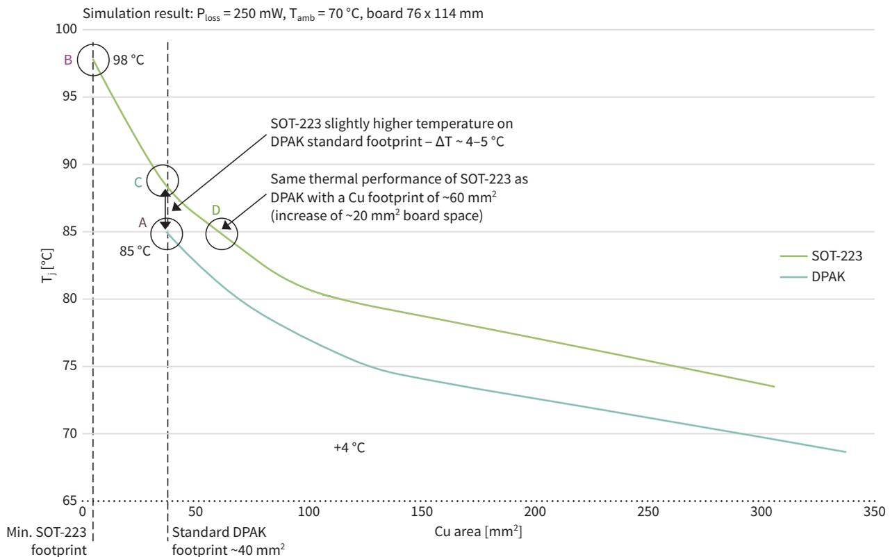
The laboratory findings on thermal behavior are confirmed by a thermal simulation with  $T_{\text{ambient}} = 70 \text{ }^\circ\text{C}$  and  $P_{\text{loss}} = 250 \text{ mW}$ . The size of the copper area in the footprint is shown on the x-axis, while the y-axis displays the temperature of the package top side. In the case of an SOT-223
