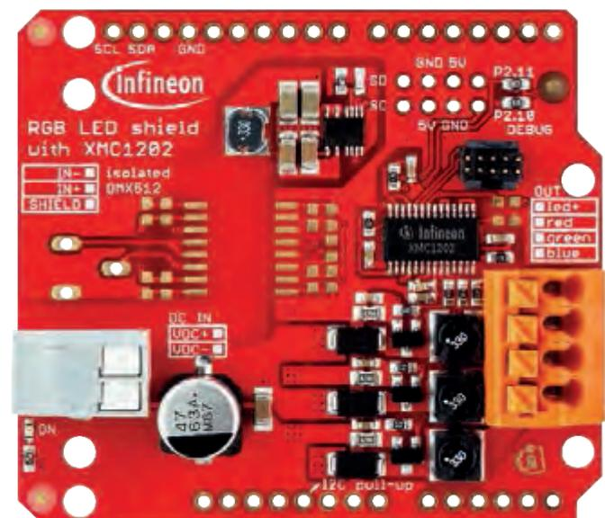
Shield can be used with an Arduino (Genuino) Uno R3 board or with the XMC1100 boot kit
