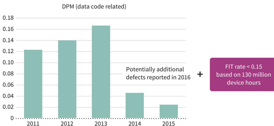
CoolMOS™ comes with a DPM of less than 0.1 and FIT rate of less than 0.15
