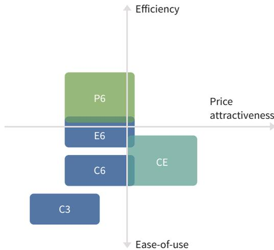
> **CoolMOS™ CE** is a general-purpose series, available in 500 V, 600 V, 650 V, 700 V and 800 V, that is optimized for the best balance between cost, efficiency and ease-of-use. We recommend the CE series as the first choice for cost-sensitive LED lighting applications for diverse topologies.
