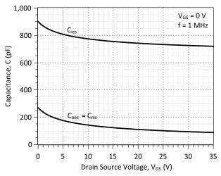
Figure 7: Typical Capacitance vs Drain-Source Voltage
