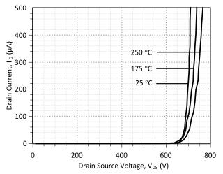
Figure 6: Typical Blocking Characteristics
