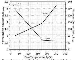
Figure 5: Normalized On-Resistance and Current Gain vs. Temperature
