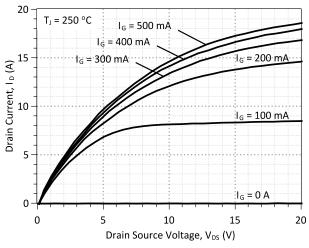
Figure 3: Typical Output Characteristics at 250 °C
